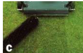
C Grooming reel designed to remove thatch in the upper layers 39 spring steel blades with 13 cutting tips at 12mm blade spacing
