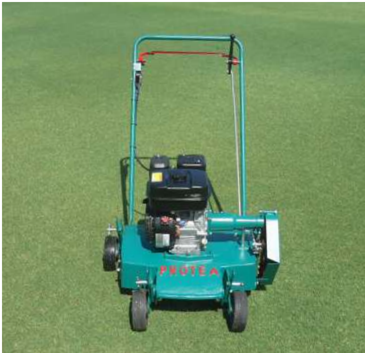
B Pin-type Scarifying Reel for aggressive treatment and removal of damaged turf.
