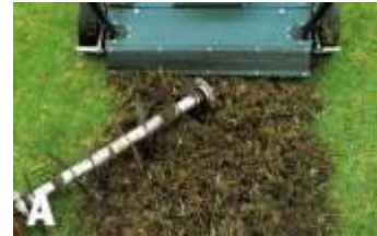
A Offset Scarifying Reel for use on fine turf to remove thatch 10 spring steel blades with 2 cutting tips at 50mm spacing
